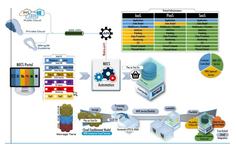
The NECS Automation REST API provides consumer, administrator, and provider-level access to the service catalog with the same services that support the NECS Cloud Management Portal (CMP) user interface. You can perform NECS Automation functions programmatically by using REST API service calls.
